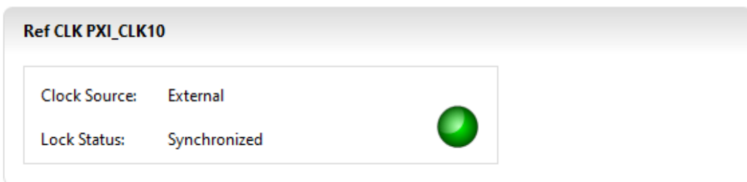
Figure 18 Reference Clock Status Display for external clock source
